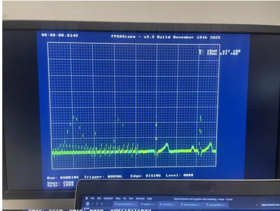
This bug has happened when experimenting with a dynamic buffer size, the issue was that for every increase of the time-scale less data would be able to be displayed per pixel slice of the screen and so it would take smaller and smaller portions of the screen from the left hand side, hence you can see the most zoomed in section on the left.
